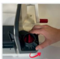
8. To release the red lock for the cutting thickness, move it to position **1**. Then set desired slice thickness (0 – 26 mm) using the thickness ring.
